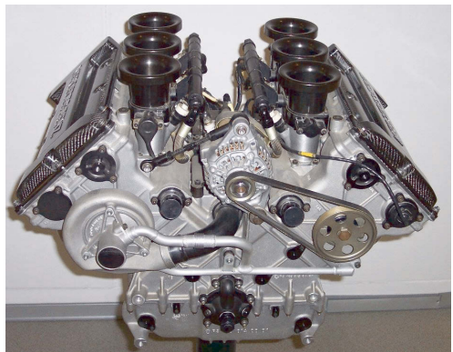
Figure 2: A complicated system: a V6 internal combustion engine from a Mercedes car (source: Wikipedia).
