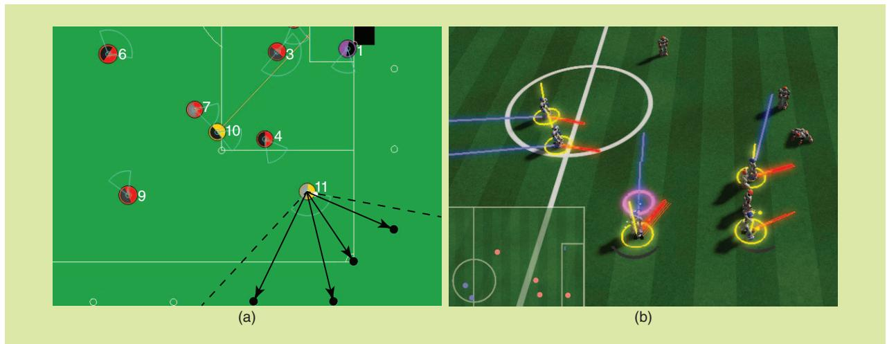
**Figure 1.** An example of screenshots from the RC simulation leagues: (a) 2-D [5] and (b) 3-D [1]. The 2-D simulation league screenshot demonstrates players from two teams (represented by red and yellow circles) and their respective fields of view. The black arrows around player 11 illustrate how an agent can self-localize from observations of unique landmark features [12]. The 3-D simulation league screenshot demonstrates similar tactical overlays for each player.
